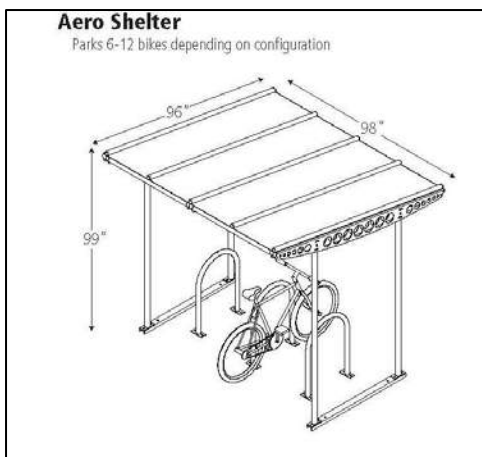
Figure 5.5. Example of a modular, pre-fab bicycle shelter manufactured by DERO.
