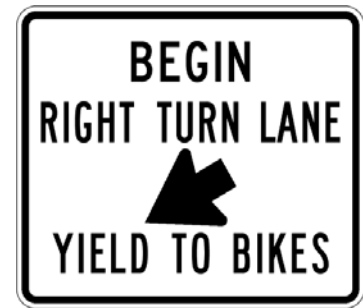
Figure 3.9. Regulatory signage for motorists to raise awareness of bicyclists and pedestrians at intersections. Source: http://mutcd.fhwa.dot.gov
